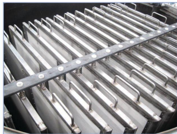
滤网在设备内部细照 Fine strainer inside the device according to the
